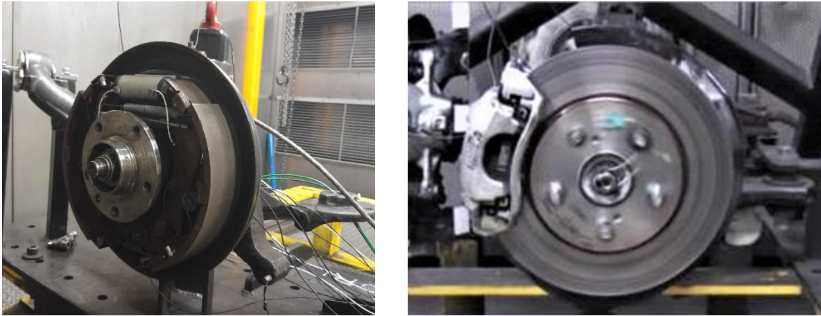
Figure 1 : Experimental setups. Left drum-brake used for section 3. Right : disk-brake used for sections 4-5.
