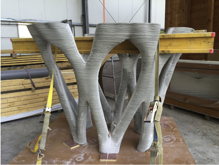
Figure 3.7 Cast and lost formwork assembly from which the printing supports were cut.
