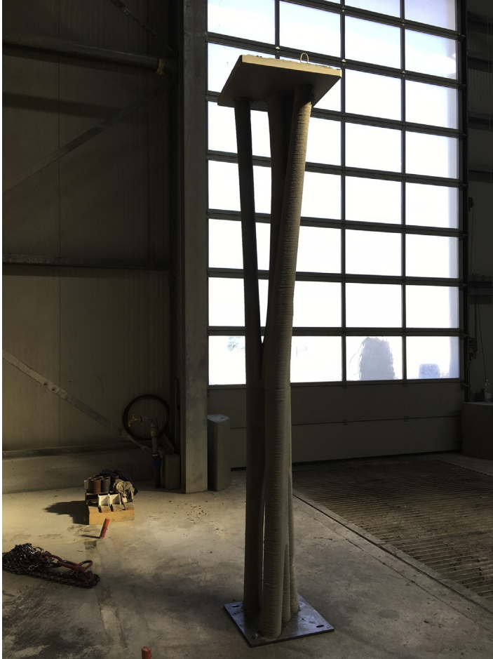
Figure 3.14 Assembled 3D-printed concrete formwork filled with UHPC casting.
