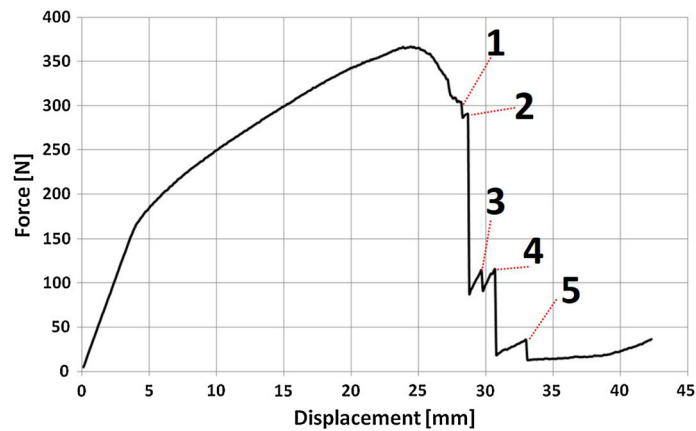
Fig. 14 Entire extensional test graph of aluminum sample A
