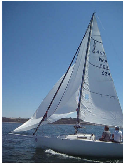
(d) Collapse of the sail if even more eased.
