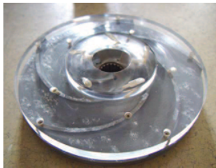
Figure 4. DERAP impeller picture and geometric specifications.
