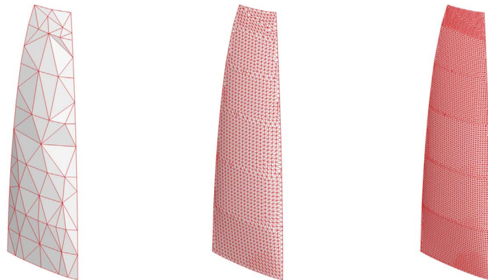
(a) \approx 100 membrane elements. (b) \approx 2,700 membrane elements. (c) \approx 9,000 membrane elements.
