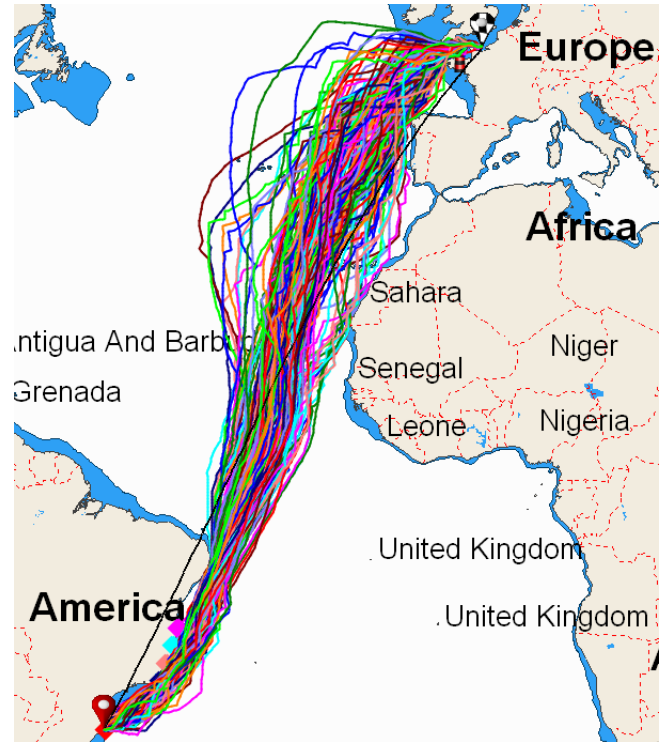
Fig. 6. Statistical routings for the Jacques Vabres 2015 race for an IMOCA60. Calculations are based on meteorological data for the past 10 years for 150 departure dates with a range of \pm 7 days.
