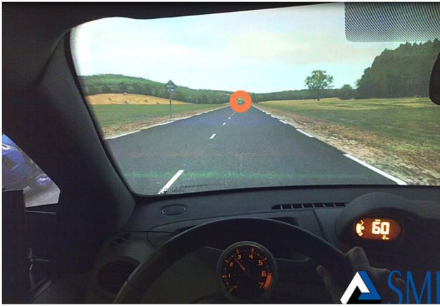
FIGURE 5 Calibration pattern for eye tracking.
