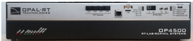
Fig. 10. HIL hardware, model OP4500 from OPAL RT technologies, used to simulate the faulty induction motor model in real time.
