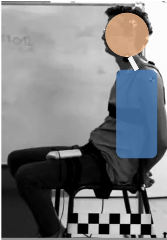
Figure 1. Simplified representation of the 3-body model superimposed on the initial neutral position of one volunteer on the sled in the experiment.
