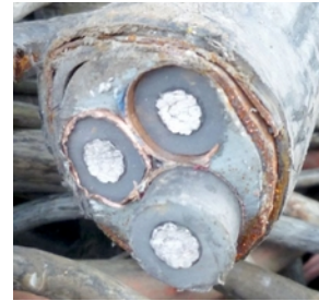
Fig. 2. Section of multiple aluminum beams cable
