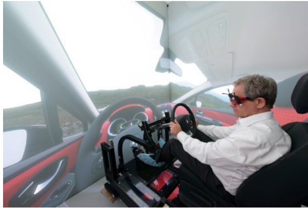
Figure 1 - Renault's High Performance CAVE with controlled driver station
