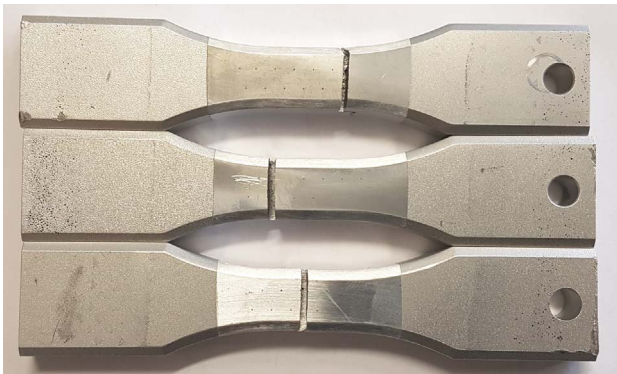
Fig. 9. Initiation site randomly located on 3 specimens containing 22 defects of Ø200 µm (specimens D200-22-1, D200-22-2 and D200-22-3).
