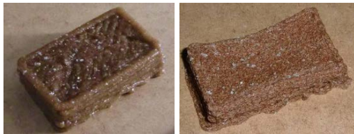
FIGURE 2. Test samples produced using wood pulp.
