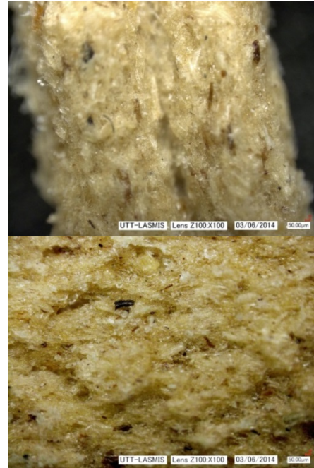
FIGURE 4. Microstructure of two wood filaments (a) and fibers size (50 \mu\text{m} scale X 100) (b).
