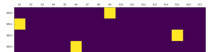
Fig. 13. Best robot allocation to the workstations minimizing completion time for assembling EBs ( Y^* ).
