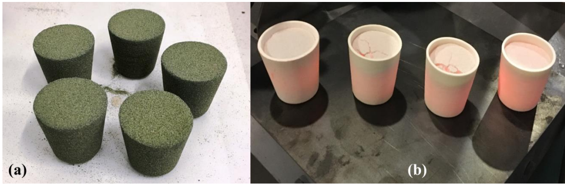
Figure 3: LOI test with (a) 3DP specimens, (b) immediately after taking out of the oven at 900 °C
