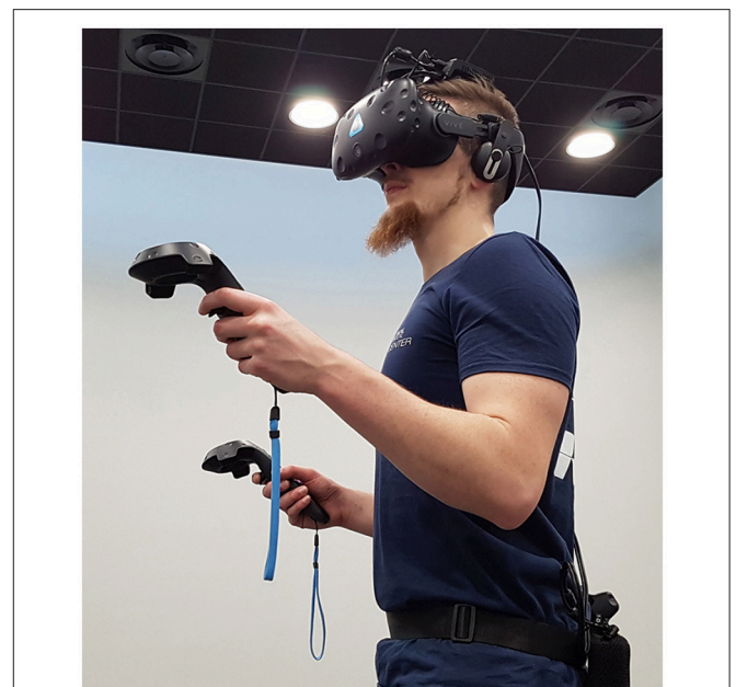
FIGURE 4 | User equipped with the required devices for the experiment: HTC Vive virtual reality headset, Vive trackers, TP Cast wireless adapter. Written informed consent was obtained from the depicted individual for the publication of this image.
