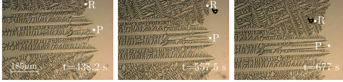
(c) Elimination of a branch at a converging grain boundary.
