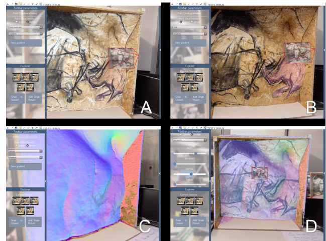
Figure 4: Very first results of AR visualization of an Aioli project with the Chauvet-Pont d'Arc facsimile. A: Dense point cloud. B: Sift cloud and dense annotation point cloud. C: Dense point cloud with normal texture. D: Composite texture (RGB and Normals).
