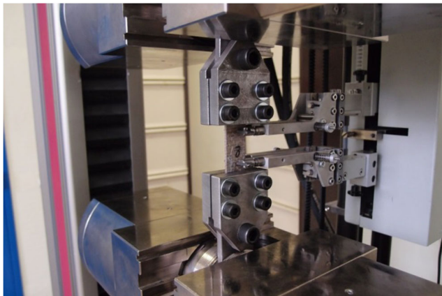
Fig. 7 Specially developed tensile test holders for non-standard samples
