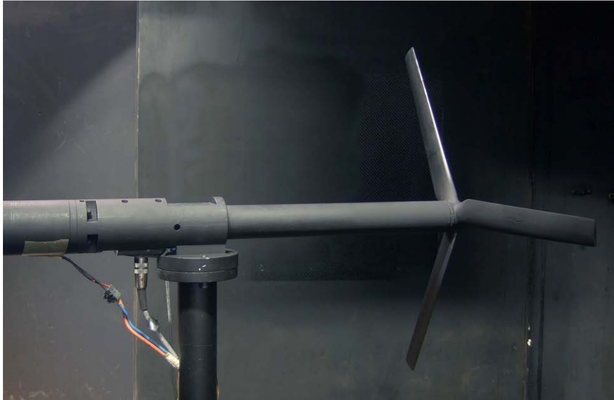
FIG. 15: Tested wind turbine in the wind tunnel
