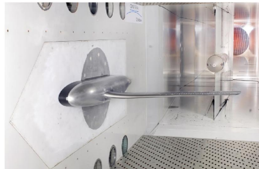
b) AVERT model in S2MA wind tunnel
