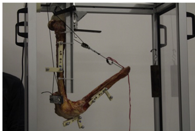
Figure 1. View of the device used to set in motion the knee specimens. The clusters of markers fixed to the femur, tibia and patella bones are also depicted.
