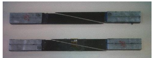
Figure 8 10^\circ Shear failure
