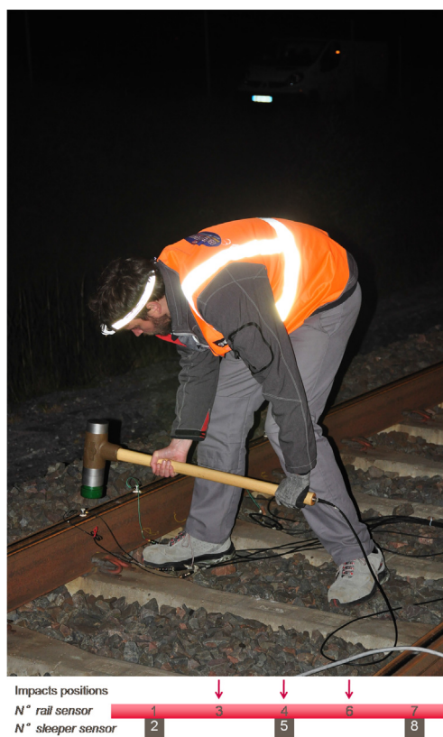
Fig. 13. Experimental setup for receptance tests in Chauconin transition zone test site.
