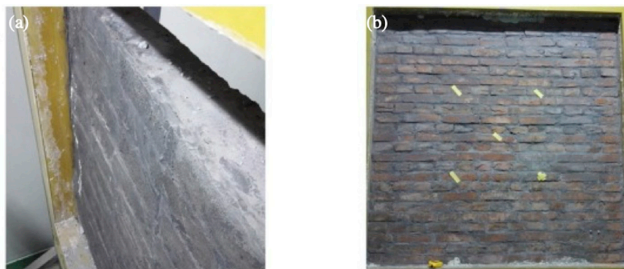
Fig. 12. An overview of the wall (a) With cPCM, and (b) Without cPCM [120]. Copyright (2019), with permission from Elsevier.
