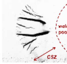
Figure 8 Illustrated CSZ length measured in cracked mushy zone after Varestraint test.
