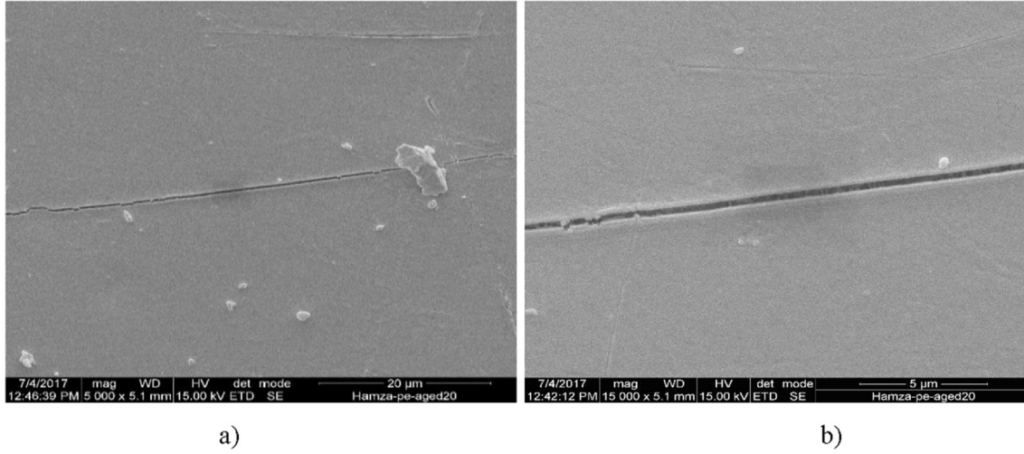
Fig. 7. SEM micrograph of an irradiated surface (20 h): (a) cracks network; (b) magnified view of a crack.
