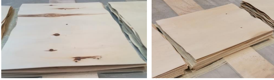
Figure 3. Veneers used in the paneling process. Left: Low quality veneers for Q2 panels. Right: High quality veneers for Q1 panels.
