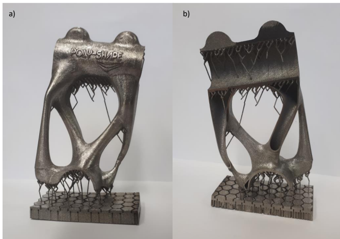
Figure 15: The Stem test case printed in LBM
