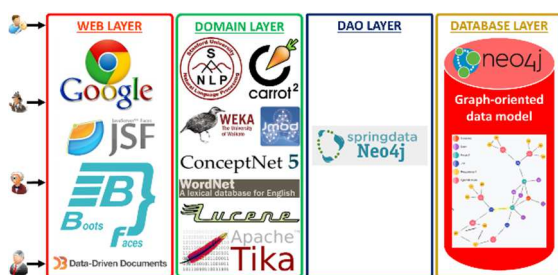
Fig. 7. Architecture of the JAVA Web application prototype
