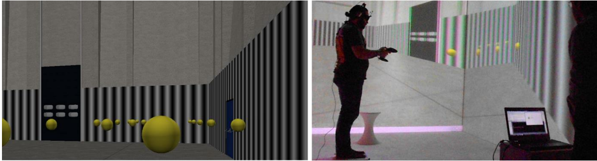
Fig. 4 Left: virtual environment displayed in the CAVE from the subject's viewpoint. Right: subject performing the experiment.
