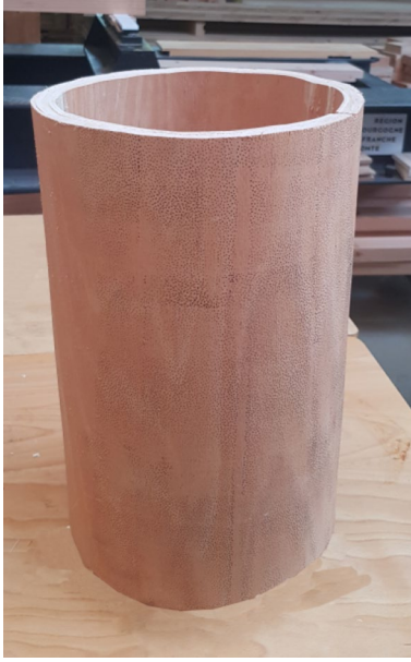
Fig. 2 Circular hollow tube made of green beech veneer
