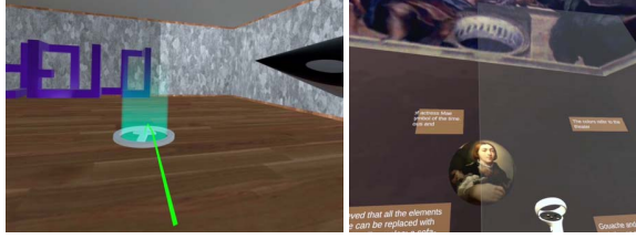
Figure 2: Left: teleportation with view orientation and parabolic target. Right: the spinning wheel interaction.
