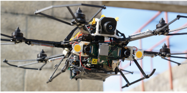
Fig. 20. Firefly UAV equipped with the VI sensor [41].
