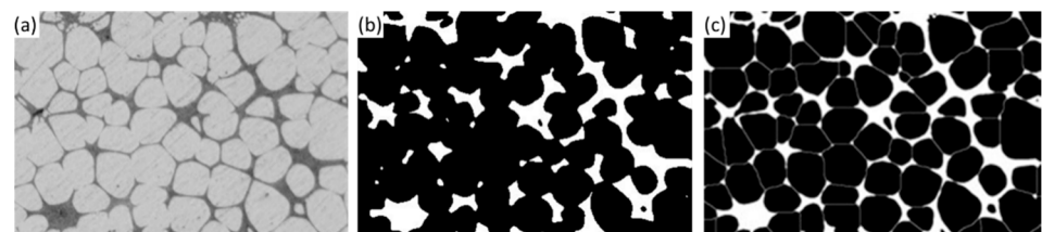
Figure 2. Segmentation of optical micrographs using a thresholding-based histogram algorithm. (a) Optical micrograph showing brighter solid grains and darker liquid phase; (b) binary image where black areas correspond to liquid phase; (c) grain boundaries identification by watershed segmentation method.
