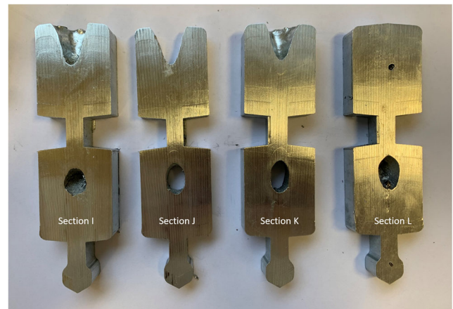
Fig. 12 Pictures of some planes showing macro-shrinkage formation
