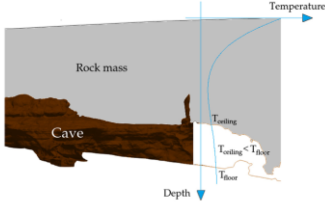
Fig. 4. Typical temperature profile in a rock mass resulting from conductive heat transfer. The downward temperature gradient stemming from the ceiling temperature which becomes colder than the floor temperature ( T_{\text{ceiling}} < T_{\text{floor}} ) can lead to the onset of thermal convection.
