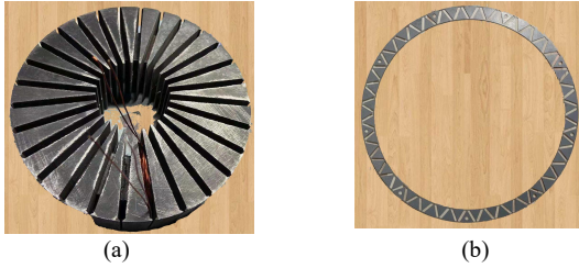
Fig. 7. Prototype with (a) Stator in SMC and (b) laminated radial rotor
