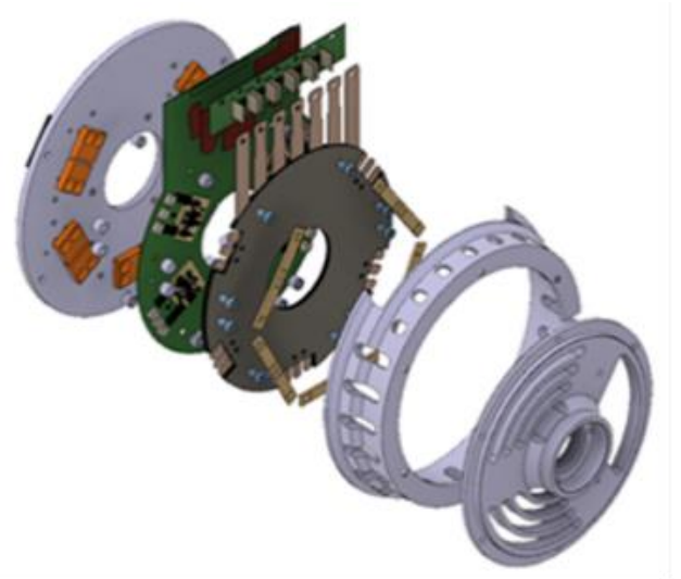
Figure 16 exploded view of one VSI with five-leg for prototype 1
