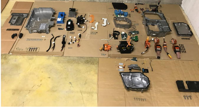
Fig. 3. Junction box after complete disassembly.
