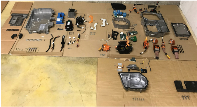
Fig. 3. Junction box after complete disassembly.
