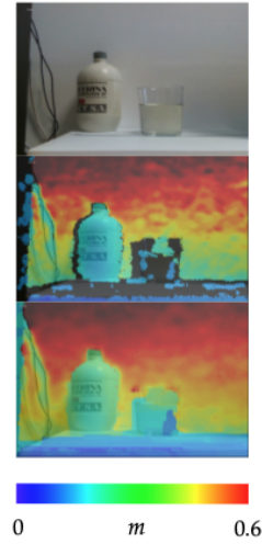
Figure 7: Color and depth stream before (up) and after (down) applying the required filters to reconstruct the depth map of the streaming.
