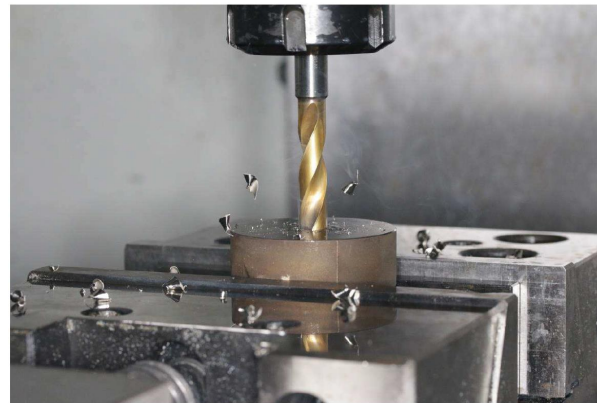
Figure 3. Experimental setup during the dry drilling tests.
