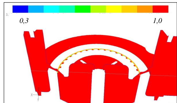
Fig. 9. Contours of volume fraction of water with a cavitation model (FLUENT).
