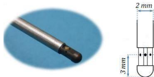
Figure 1: picture and sketch of the three-hole pressure probe
