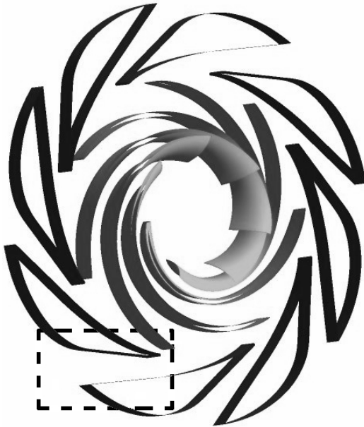
Figure 1 Schematic representation of the centrifugal pump. The dotted line indicates the investigated diffuser blade passage.
