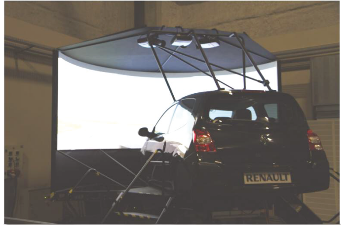
Figure 17. Operating of the dynamic driving simulator SAAM
