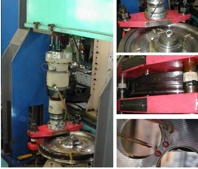
Fig. 14. Drilled wheel on SNCF-AEF fatigue test bench.
