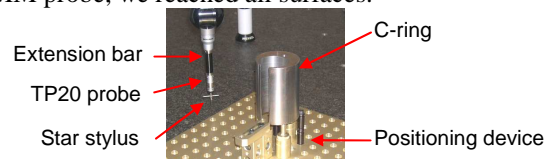
Figure 3: C-ring test part and its measuring device
