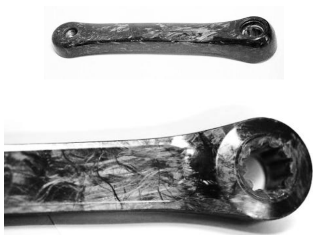
Figure 7. Natec pedal crank Desired characteristics: specific stiffness and equivalent mass to the classic one (approx. 185 g)
